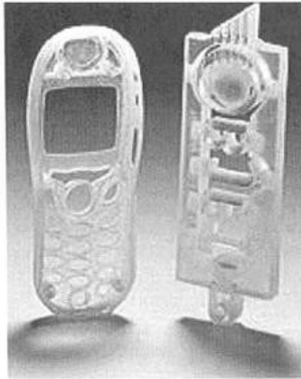
Figure 6.2 Parts built with the Objet Quadra photocurable resin.
