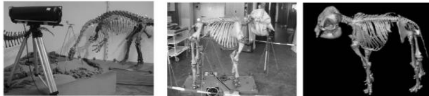
Figure 8: Left: scanning setup (Laser Scanner Menzi S25 ) with dinosaur skeleton and reference points. Center and right: scanning setup and measured 3D point cloud of the Juvenile Indian elephant skeleton of the zoological museum of Copenhagen (Denmark).
