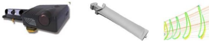
Figure 7: Optical 3D digitizer Nub3D Triple (Spain) (left); measured turbine blade (center); profile analysis (right).
